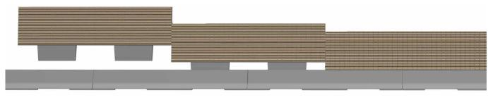
The REBLOC® Integrated Noise Barrier consists of a base element of New Jersey profile and a plateshaped noise barrier element. The slim total system width makes optimum use of the space available. One noise barrier element is inserted overlapping
